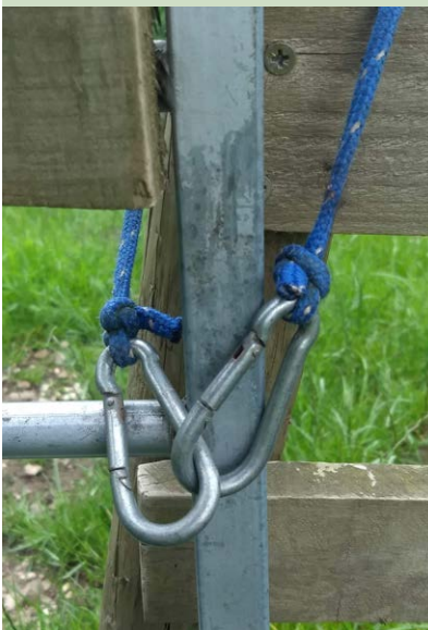
Figure 34. A pair of snap hooks on a piece of rope makes a versatile quick-release fastener.
