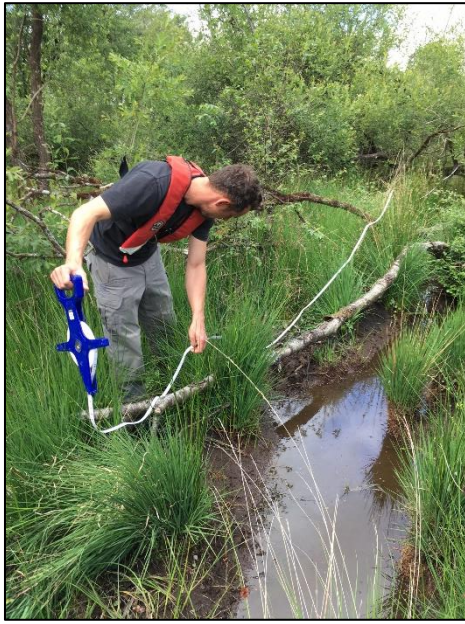
Figure 9: Width and height measured within the enclosed beaver site in the headwaters of the Tamar
